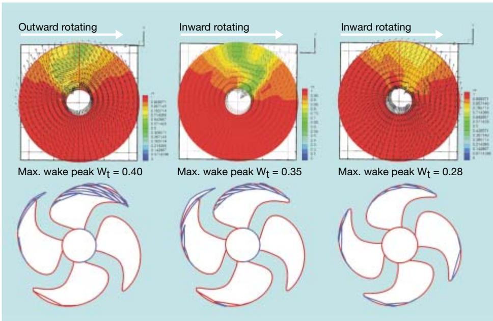
**Fig. 4 Effect of wake fields on direction of rotation and calculated cavitation extent for fast RoPax vessel.**
