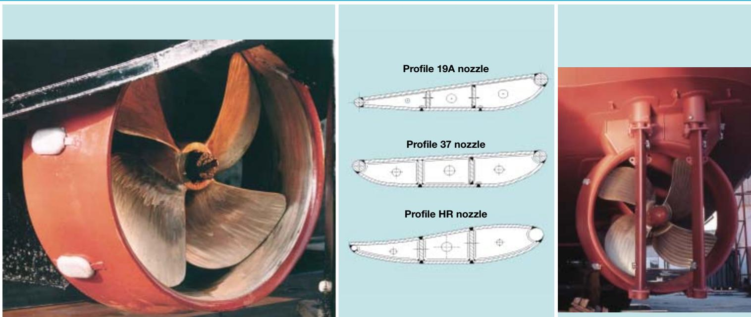
Fig. 11 Examples of propeller nozzles used by Wärtsilä.
