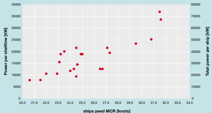
Fig. 2 Power per shaft versus ship speed for RoPax vessels.
