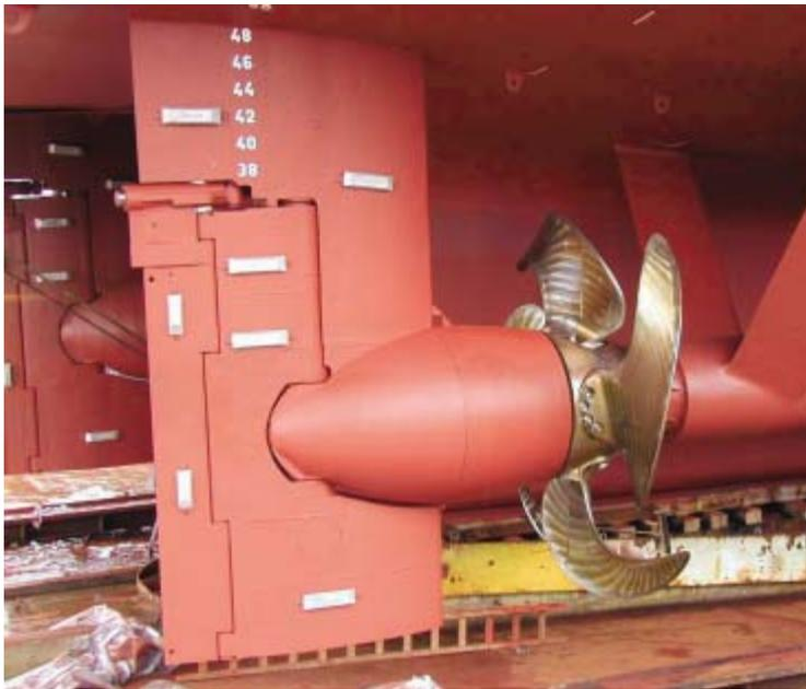
Fig. 9 The Efficiency Rudder on a twin-screw vessel.
