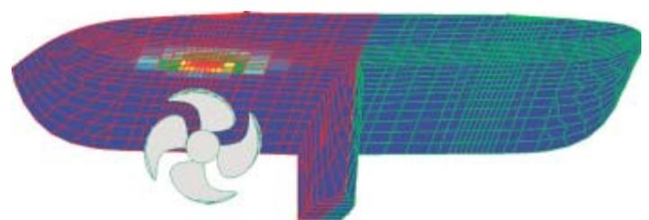
**Fig. 6 Integration of pressure pulses on the hull as input for vibration analysis.**
