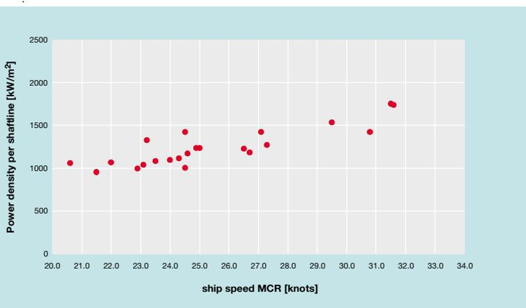
Fig. 3 Power density versus ship speed for vessels.
